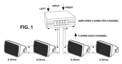
Be sure to use a good quality, unshielded twisted pair speaker cable to connect the amplifier to the speaker(s) (#14AWG for runs <80', #12AWG for runs >80'). Standard ZIP style speaker cable may also be used if twisted pair cable is not available.
